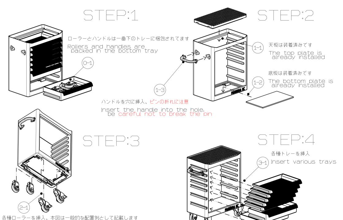
Various rollers are inserted, and this figure is shown as a general layout example.
